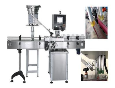
Cap diameter: 20 - 80mm. Bottle diameter: 90mm Max. Bottle height: 300mm Max.
